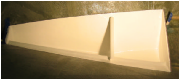
Auxiliary water tank under construction
