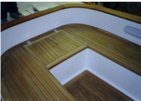
The seat hatches have fiberglass drains integrated into the perimeter to keep locker contents dry
