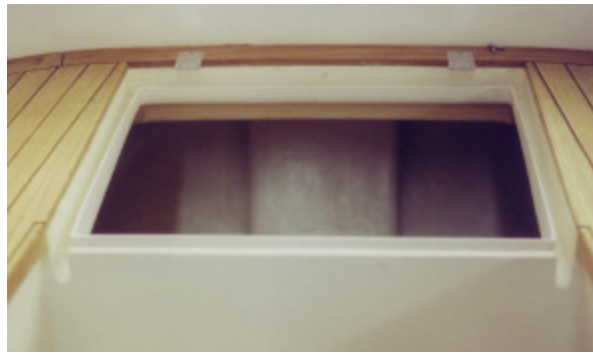
The seat hatches have fiberglass drains integrated into the perimeter to keep locker contents dry
